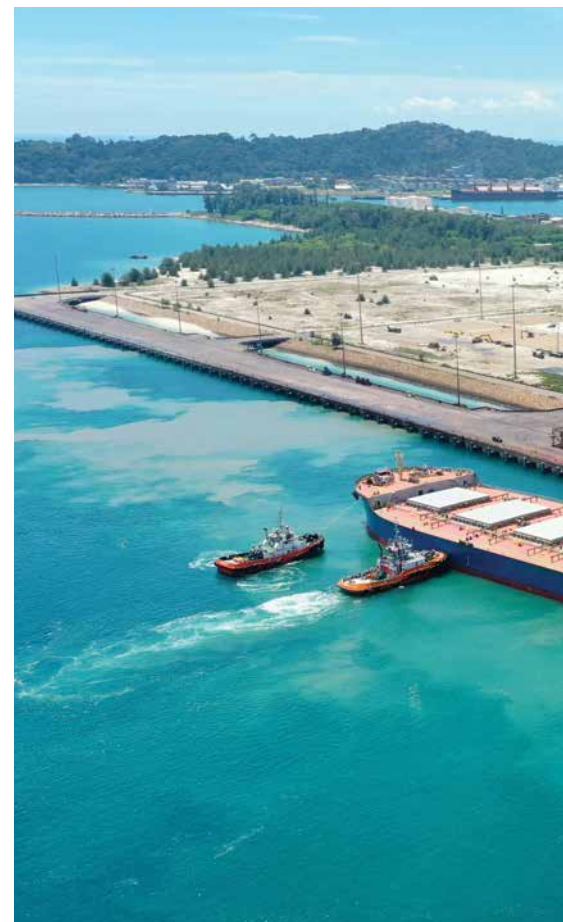
MV Heng Mao, the deepest vessel ever berthed at Kuantan Port, with a 16.4-metre draught
