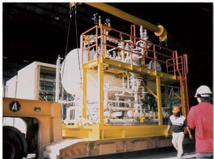
Loading of 'Produced Water Package' for Offshore Process Module
